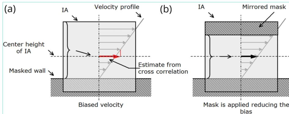
**Figure 1** (a) IA without wall correction results in overestimated velocity. (b) Flow masking reduces the bias.
